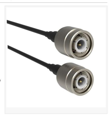
TNC cable assemblies utilize high-quality TNC connectors which feature a threaded coupling mechanism for secure mating and stable performance. These connectors are manufactured from brass with nickel plating and offer reliable electrical performance up to 11 GHz, or to the limits of the cable type. Additional cable options now include RG-58, RG-142, RG-316, and Times LMR-195.
