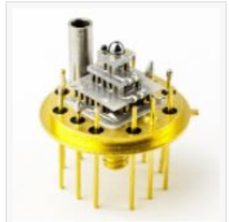
MWIR InAsSb Sensors / Detectors with cooling to improve pweformance
