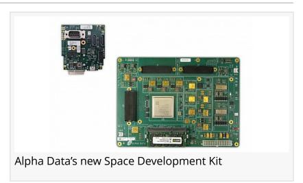
that look to incorporate the Xilinx™ Radiation Tolerant Kintex® UltraScale™ XQRKU060 Space-Grade FPGA.
