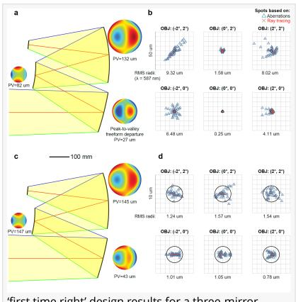
'first time right' design results for a three-mirror imager: a&b - directly calculated initial system; c&d subsequently optimized final system.
