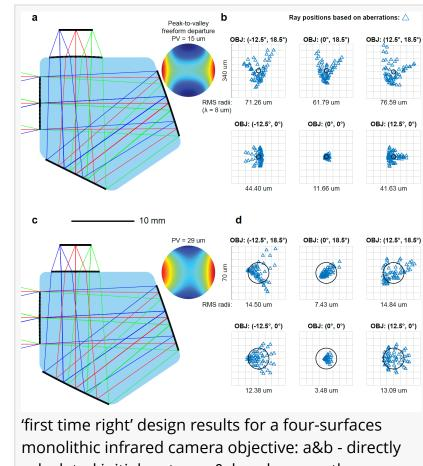
monolithic infrared camera objective: a&b - directly calculated initial system; c&d - subsequently optimized final system.
