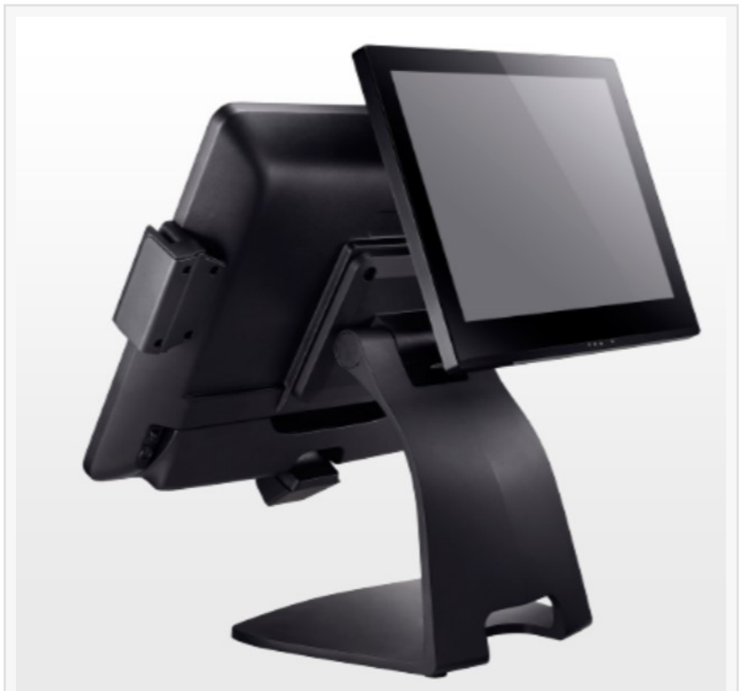
Optional VFD or 8" or 9.7" bezel-free customer-facing display
