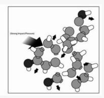
The higher degree of entanglement means that in order to rupture, more polymer bonds need to be broken. At high impact, the external kinetic energy cancels out with this intermolecular force, and virtually "absorbs" the force that can hurt the person.
