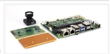
congatec i.MX 8M Plus starter set for AI accelerated embedded vision applications
