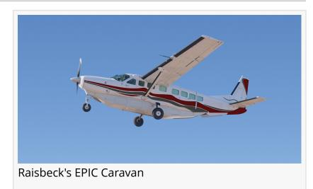
the comprehensive pre-certification flights tests marks a significant milestone and clears the way for STC approval which the company anticipates receiving in August. The system includes a composite Forward Cargo Pod Fairing and metal Dual Aft Body Strakes.
