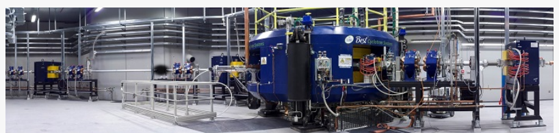
Best 70 MeV Proton Cyclotron installed in INFN, Legnaro, Italy (Photo courtesy of Laboratori Nazionali di Legnaro)
