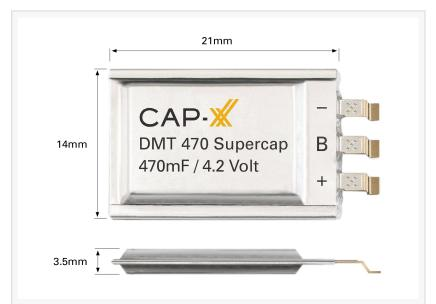
Thin prismatic CAP-XX DMT470 supercap fits easily inside the small (7.4cm x 7.4cm x 5.6cm) sensors and supports the battery by storing energy and delivering burst power for data transmissions
