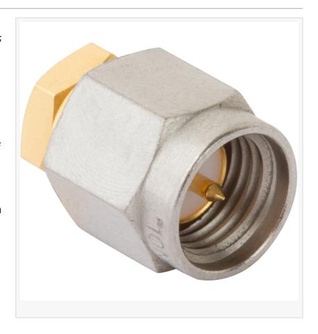
SMA connectors utilize the reliable threaded coupling mechanism as the rest of the series for easy and secure mating. They are constructed from brass with gold plating and feature an antitorque body designed to reduce stress on cable and solder joints.
