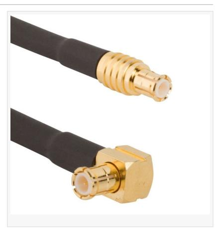
The MCX connector series is a robust micro-miniature interface with broadband capabilities of DC to 6 GHz that feature secure snap-on/snap-off coupling for quick and easy mating. These connectors are manufactured from brass with gold plating and offer reliable electrical performance up to the limits of the cable type. Their small size paired with the flexible cable types make them an ideal choice for compact applications.
