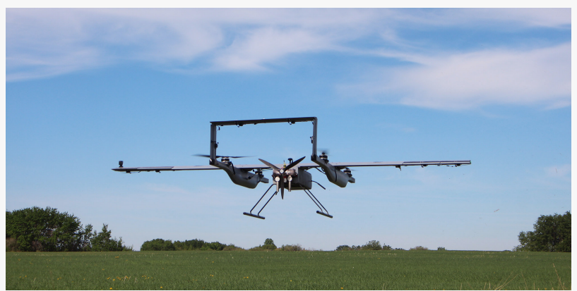
A Pegasus Imagery PV-02 Eos lifts off and takes off vertically like a quadcopter before transitioning to horizontal flight. The PV-02 Eos is a fixed-wing class III VTOL RPAS
