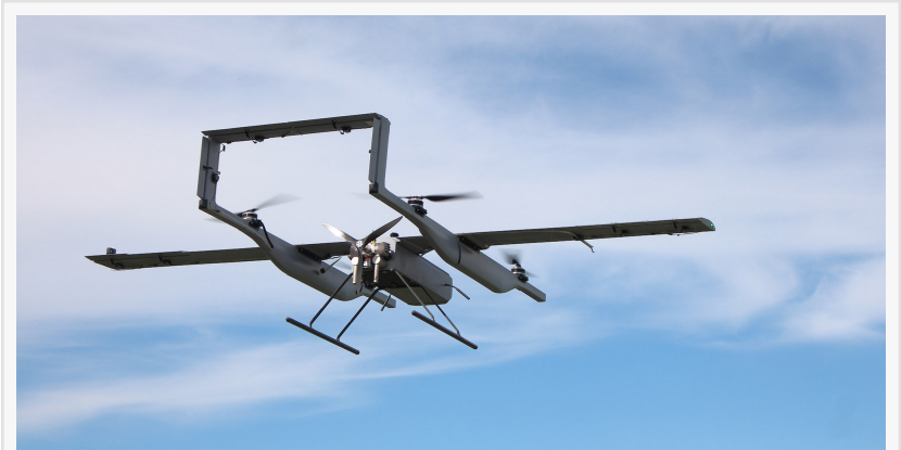
A Pegasus Imagery PV-02 is shown in flight. The PV-02 Eos is a fixed-wing class III VTOL RPAS.
