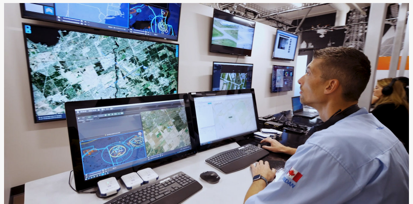
Kongsberg Geospatial's IRIS UxS combines real-time data from multiple sensors to create a real-time, 3D picture of the airspace where drones are operating.
