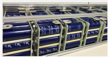
RGM's module, based on the CAP-XX 3000F, 2.85V cell can store high energy and deliver high power very quickly: 2) 15-cell submodules are connected in series, with the single 100F, 85.5V module able to store 100Wh and deliver 150KW maximum instantaneous power.
