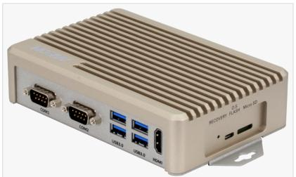
The BOXER-8230AI features flexible I/O connections, with five Gigabit LAN ports, four USB3.2 Gen 1 ports and two COM ports.
