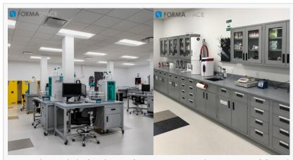
Metrohm's lab facilities feature a combination of fixed casework as well as modular (freestanding) lab workbenches mounted on heavy-duty casters, which offer maximum layout flexibility as needs change over time.
