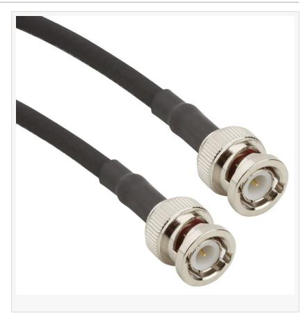
BNC cable assemblies are engineered using high-quality connectors which feature the familiar bayonet coupling mechanism for easy mating and un-mating. These connectors are manufactured from machined brass and diecast zinc with nickel plating and offer reliable electrical performance up to 3 GHz. LMR low loss cable is designed with improved shielding compared to standard RF coaxial cables which allows it to achieve low attenuation loss at high frequencies.
