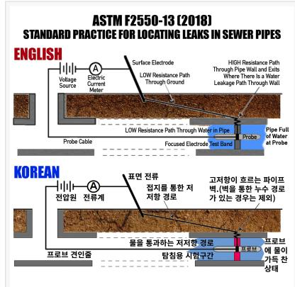
Since Acoustic Sensors and Closed Circuit Television (CCTV) cameras are unable to locate or measure leaks in gravity sewers, a new ASTM standards, first introduced in 2006, was established and used by many Smart Utilities to approve sewers as watertight.
