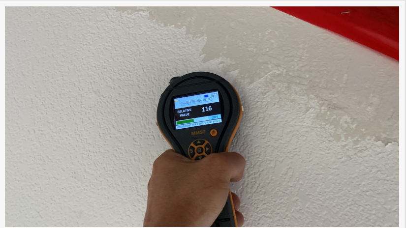
Checking the moisture level in the ceiling.
