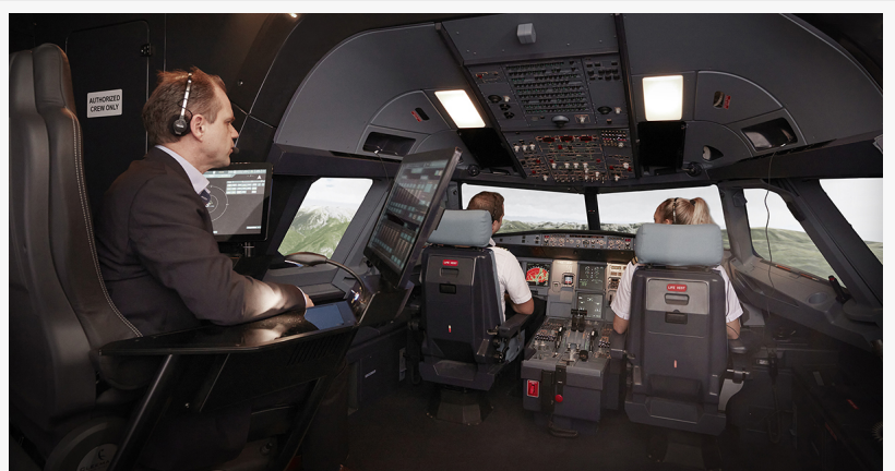
Flight training inside the Avion A320 Full Flight Simulator
