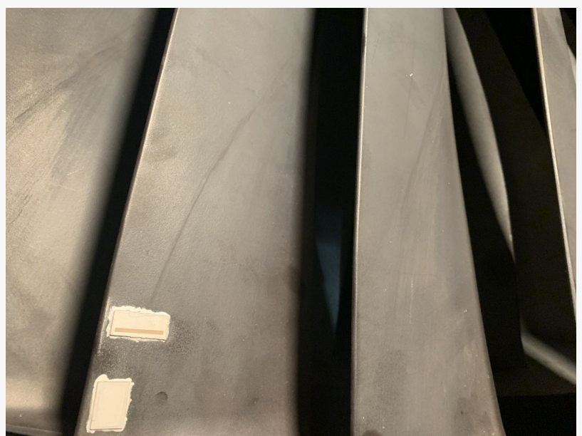
Close up image of Sensatek's passive RF temperature sensors on the blade of a gas turbine engine
