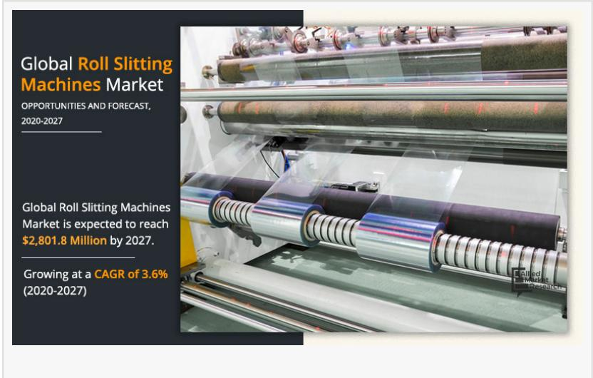
Roll slitting operation includes shear cutting of large rolls of raw materials also known as master roll or parent roll, into rolls with small and narrow shape. Roll slitting is also termed as slitting in the converting industry and plays an integral part in the flexible packaging processes.
