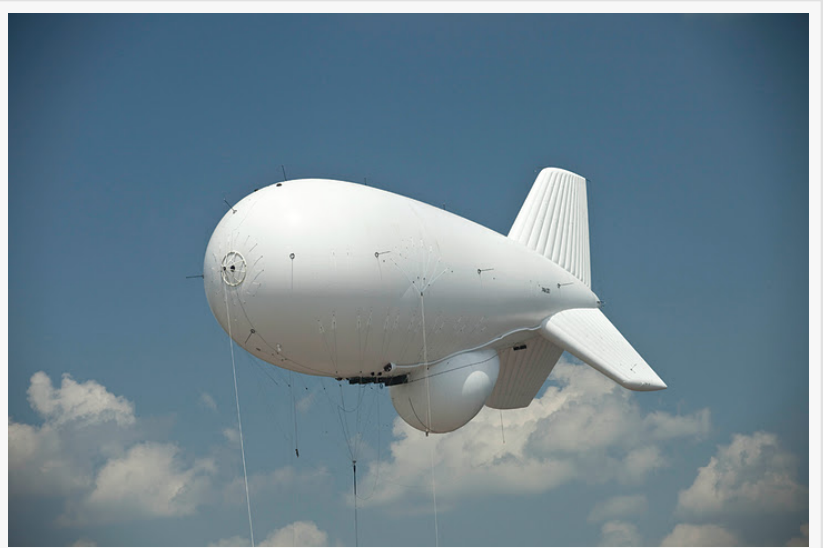
TCOM's 74M Lighter-Than-Air Aerostat ISR Platform for Persistent Surveillance
