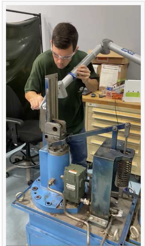
GCS Technician Michael Morel Performs Preliminary Work to Install A Woodward VariStroke Actuator
