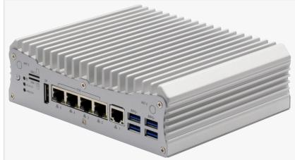
VPC-5620S Industrial System is designed to power a range of industrial edge applications with four Smart PoE ports.
