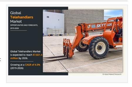
known as a telescopic handler, is a vehicle with a telescopic boom, fitted with various lifting accessories.
