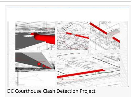
Sukh Singh, the Vice President of Tejjy Inc. said – "Our BIM Team used Revit & Navisworks software platforms for 3D Modeling of Mechanical, Electrical, Plumbing & Fire Protection services of the project. We created <u>3D Model Creation for MEPFP trades</u> for clash detection, mitigation, and visualization. Our Constructability Review through BIM Model Update helped to reflect the
