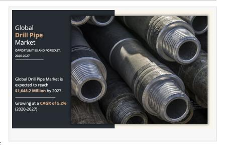
Drill pipe is a tubular steel conduit, which connects the rig surface equipment with the bottom hole assembly. The drill pipe has special threaded ends called as tool joints and it is used for pumping drilling fluid to the rig drilling bit for reducing torque generated in the pipe. A series of drill pipes is termed as drill string and the pipes are connected using different connections to maintain the length of the rig and secure the pipe joint.
