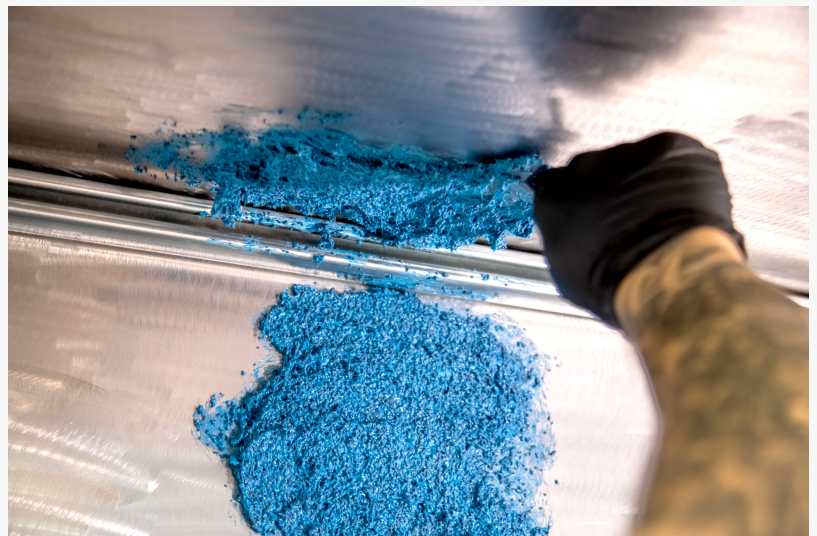
No Sag Vertical Application - Devcon Wear Guard 300RTC Compound
