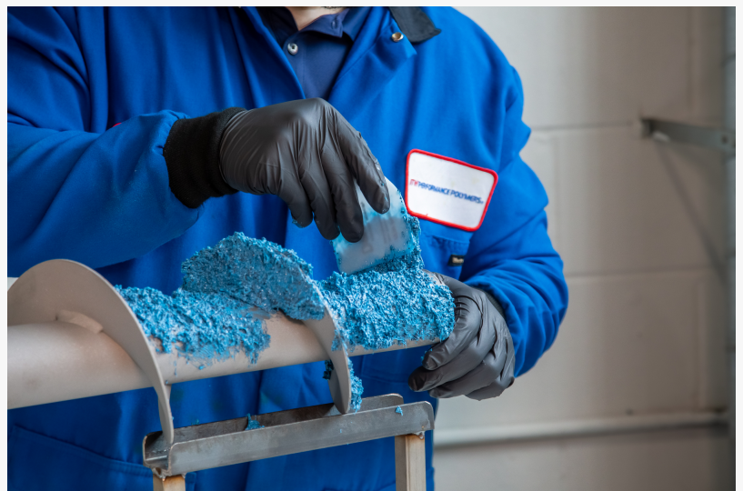
Auger Coating - Equipment Protection - Devcon Wear Guard 300RTC Compound
