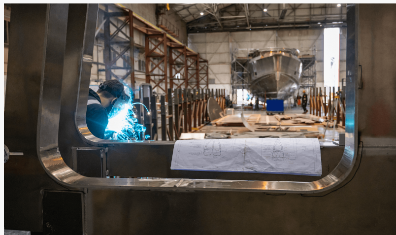
First frames of the Explorer Vessel Project Pelagos being welded into place
