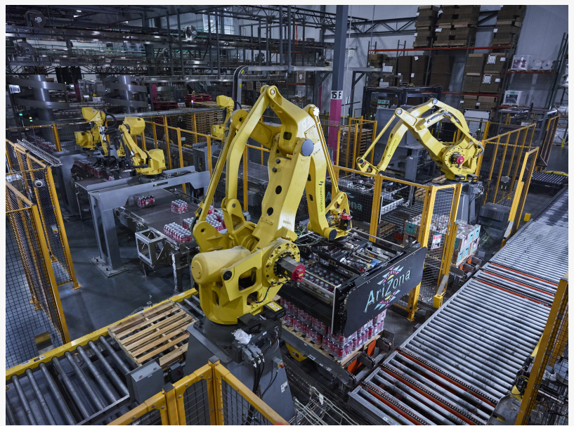
Automated material handling systems at Arizona Iced Tea's new Keasbey facility speed the processing of bottled beverage products for load staging and transport by Bettaway logistics personnel
