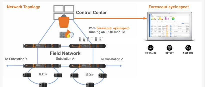
Network architecture with RAPTOR's and Forescout, eyeInspect running on the iROC module
