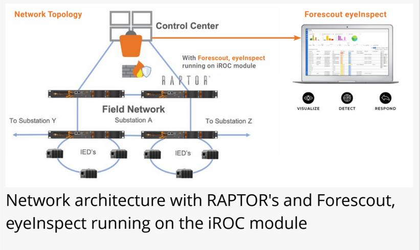
Network architecture with RAPTOR's and Forescout, eyeInspect running on the iROC module
