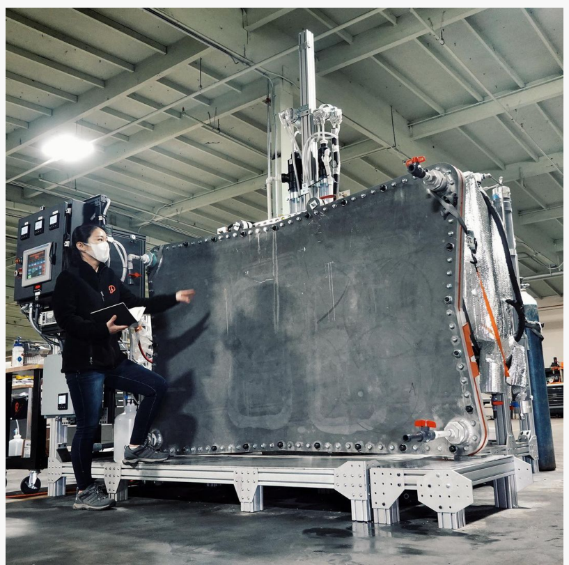
Prometheus prototype making fuel from air-captured carbon
