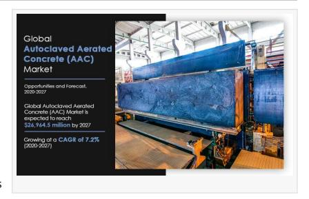
AAC is generally available as panels, blocks, and others, which can be used for wall cladding, flooring, roofing, partition walls, and others. This type of concrete mainly constitutes of around 80% air induced by the expansion agent to reduce the density and overall weight of the product.
