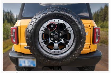
The FullVUE camera is integrated into the spare tire carrier.
