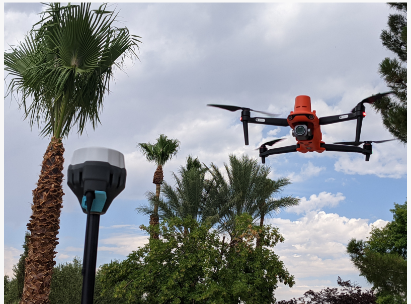
Autel RTK with Emlid GNSS Receiver
