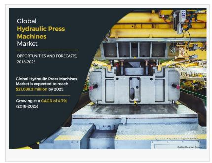
converted into kinetic energy of piston, which in turn produces shear stress between die and punch, which cuts or presses the metal. These machines are used for the for transforming metallic objects into sheets and making powders for pharmaceutical & medical industries.
