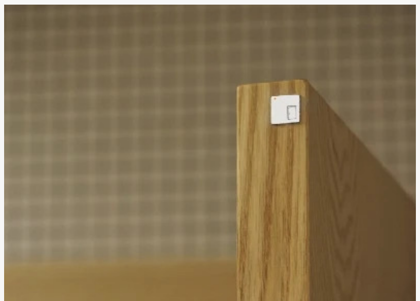
Sensors are used on restroom doors to know when and where to clean
