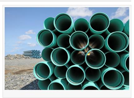
construction and electrification purposes. These pipes are resistant to chemicals and high fluid pressure which makes them fit for distribution of potable <u>water</u>. They are used for renovation and often substitute traditional materials like wood and metals. PVC pipes are not only durable and light in weight but are also cost-effective and easy to install. Their high degree of inertness and resistance to corrosion makes them an ideal choice for use in earthquake-prone areas.
