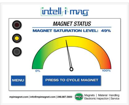
Intell-I-Mag's patented new technology uses sensors and data collection to improve analysis of magnetic separator performance, including magnet saturation, cleaning alerts, temperature monitoring, cleaning cycles and position location set by the operator,
