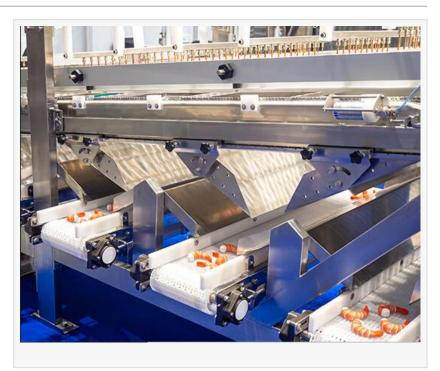
are some of the commonly used equipment. They aid in reducing wastage, improving taste, prolonging the shelf-life and minimizing the maintenance and transportation costs. Seafood processing equipment also aids in preventing enzymatic, bacterial and chemical deterioration and is widely used for the processing of mollusks, finfish and crustaceans.
