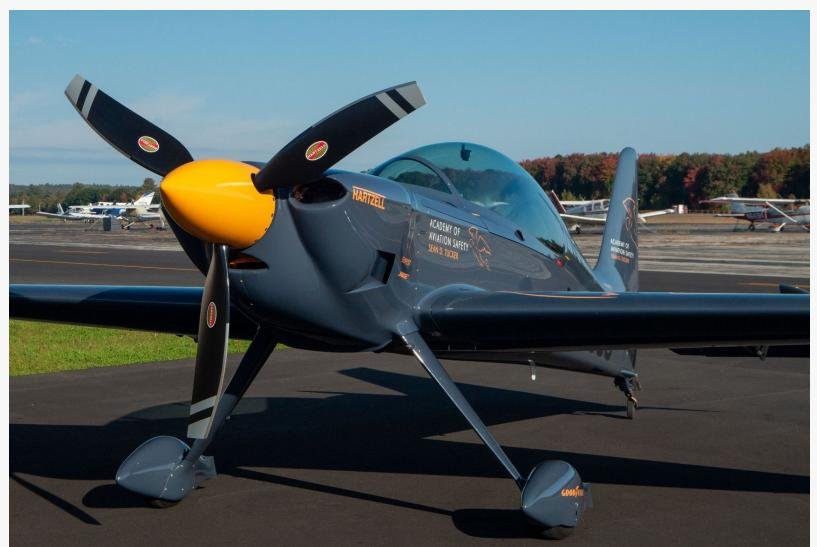
This aircraft is the first of four tandem seat GB1 GameBirds that Tucker's new formation aerobatic team will be flying on aerial demonstrations, all featuring Hartzell Talon propellers in place of factory standard equipped propellers. The all composite GB1 GameBird is an unlimited aerobic competitor, and with a 1,200 mile range it is also capable for weekend trips.
