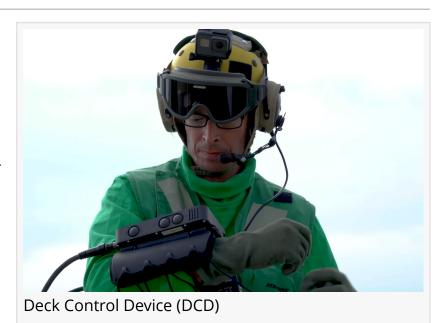
The MQ-25, designed and developed by Boeing, will be the Navy's first operational, carrier-based unmanned aircraft. The operator-worn, remote-control DCD was successfully tested earlier this
