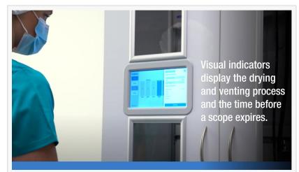
Visual indicators display the drying and venting process and the time before a scope expires.
