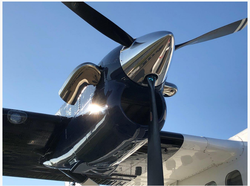
DHC-6 Next Generation Exhaust Installed on DHC-6-400 Launch Customer Aircraft
