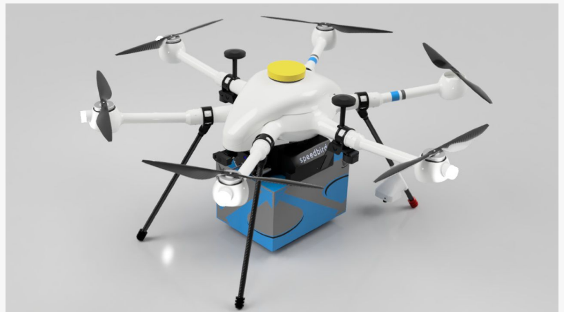
Speedbird Aero delivery drone with integrated ParaZero SafeAir parachute system
