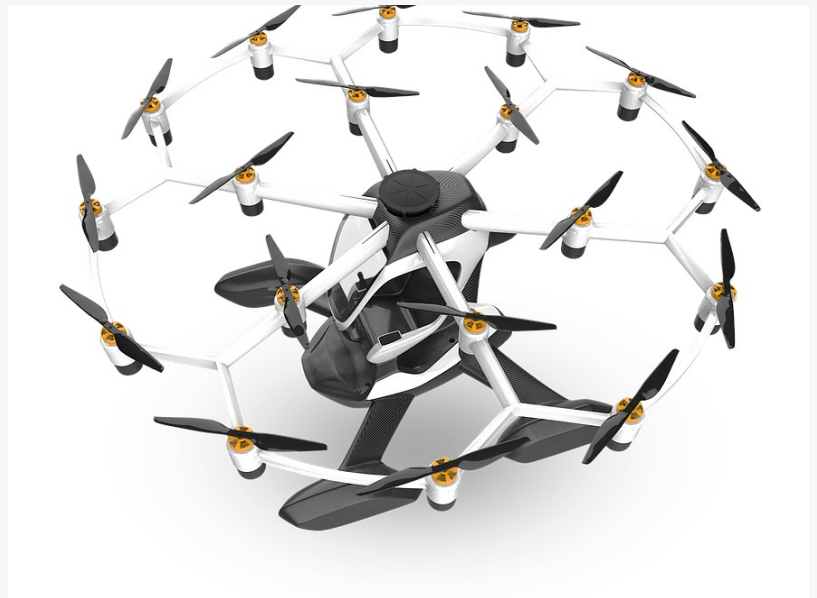
Lift Aircraft Hexa with integrated ParaZero parachute recovery system
