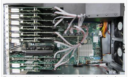
Top view: Nine M2p-cards in one PC, synchronized with the help of the Star-Hub module (in the middle). The Star-Hub can be mounted on a card as extension (like here) or as top-mount (results in 2 slots width).
