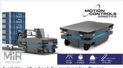
Available with a hook for towing jobs - Towing capacity: 500 kg / 1100 lbs
