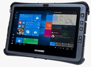
The U11 rugged tablet is MIL-STD-810H certified, ANSI 12.12.01 C1D2 certified, and IP65 rated, assuring shock, 6-foot drop, and vibration protection, as well as the ability to withstand use in a wide range of temperatures.
