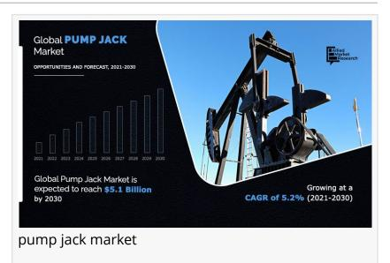
reciprocating motion to drive the pump shaft to lift up oil from oil wells. Pump jacks are commonly used in oil rich matured fields in onshore locations. Pump jack produces or lifts up generally 5 to 10 liters of liquid at each stroke depending on the size of the pump. Pump jacks offers benefits such as low operational cost, remote operation, easy maintenance, efficient extraction & production, and others.
